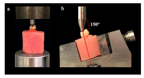
Figure 1 Position of a specimen in the test setup for static axial (a) and palatal oblique (b) loading.
