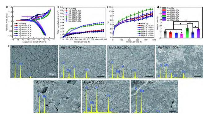
Figure 2 Biodegradation behavior of Mg-Li-Ca alloys. (a) Potentiodynamic polarization, (b) total hydrogen evolution. (c) pH of Hank's solution. (d) Weight loss of Mg-Li-Ca alloys. \*p<0.05. (e) Surface morphologies detected after 20 d immersion in Hank's solution.
