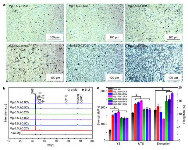
Figure 1 Microstructures and mechanical properties of Mg-Li-Ca alloys. (a) The optical images of the cross-section perpendicular to the extrusion direction. (b) XRD results. (c) Tensile yield strength (YS), ultimate tensile strength (UTS), and elongation values of the as-extruded Mg-Li-Ca alloys. \*p<0.05.
