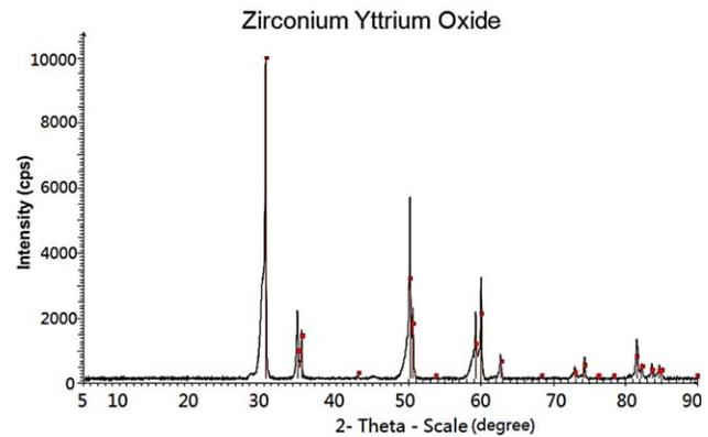
**FIGURE 3.** X-ray diffraction spectrum of zirconia disks. Its accordance with zirconium yttrium oxide. [Color figure can be viewed in the online issue, which is available at [wileyonlinelibrary.com](http://wileyonlinelibrary.com).]
