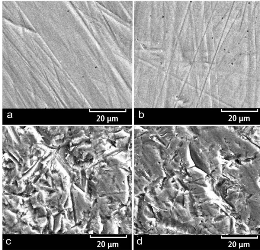
**FIGURE 1.** Surface morphology of four groups of zirconia as SEM images: (a) S-C surface, (b) S-UV surface, (c) R-C surface, and (d) R-UV surface.
