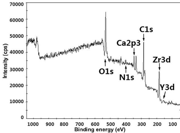
FIGURE 4. XPS spectrum of zirconia disks.
