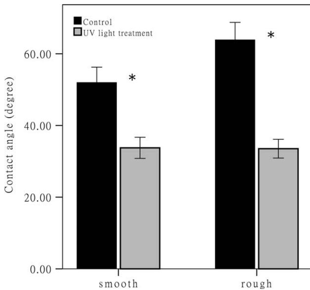
**FIGURE 2.** After UV light treatment for 24 h, the surface contact angles significantly decreased. Data are shown as mean  $\pm$  SD ( $n = 15$ ); \* $p < 0.05$ .
