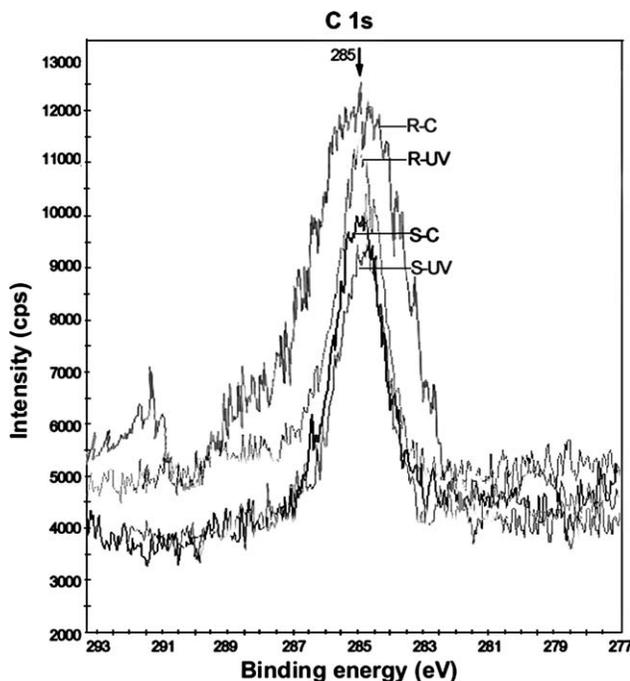
FIGURE 5. The XPS C1s peak of four surfaces. After UV light treatment the peak decreased.
