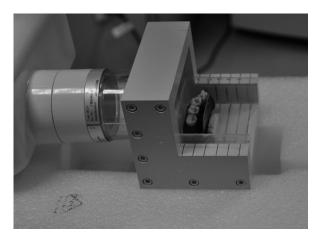
Fig. 1. Photo of a specially designed holder that enables standard projection geometry.
