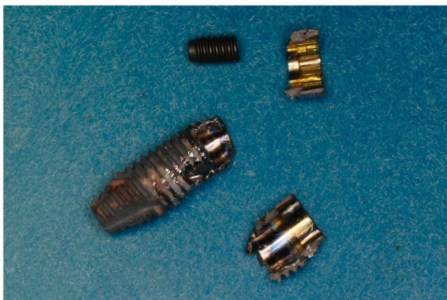
Fig. 4. Fractures at the self-tapping thread.
